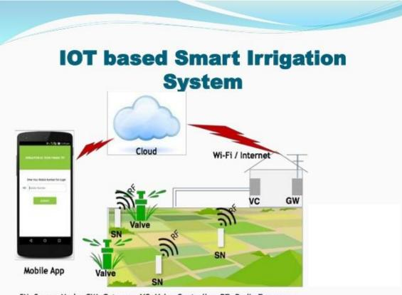
SN: Sensor Node; GW: Gateway; VC: Valve Controller; RF: Radio Frequency
